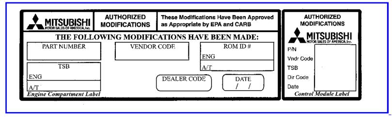
16. Carefully remove all dirt and oil from a vacant area near the VECI label on the underside of the hood, and affix the Engine Compartment label.
