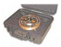
This tool supersedes T/N 07YAC-PHM010B. It's actually the same tool, but the foam insert now includes a circular cutout that makes it easier to store the heavily magnetized motor rotor after removal.
